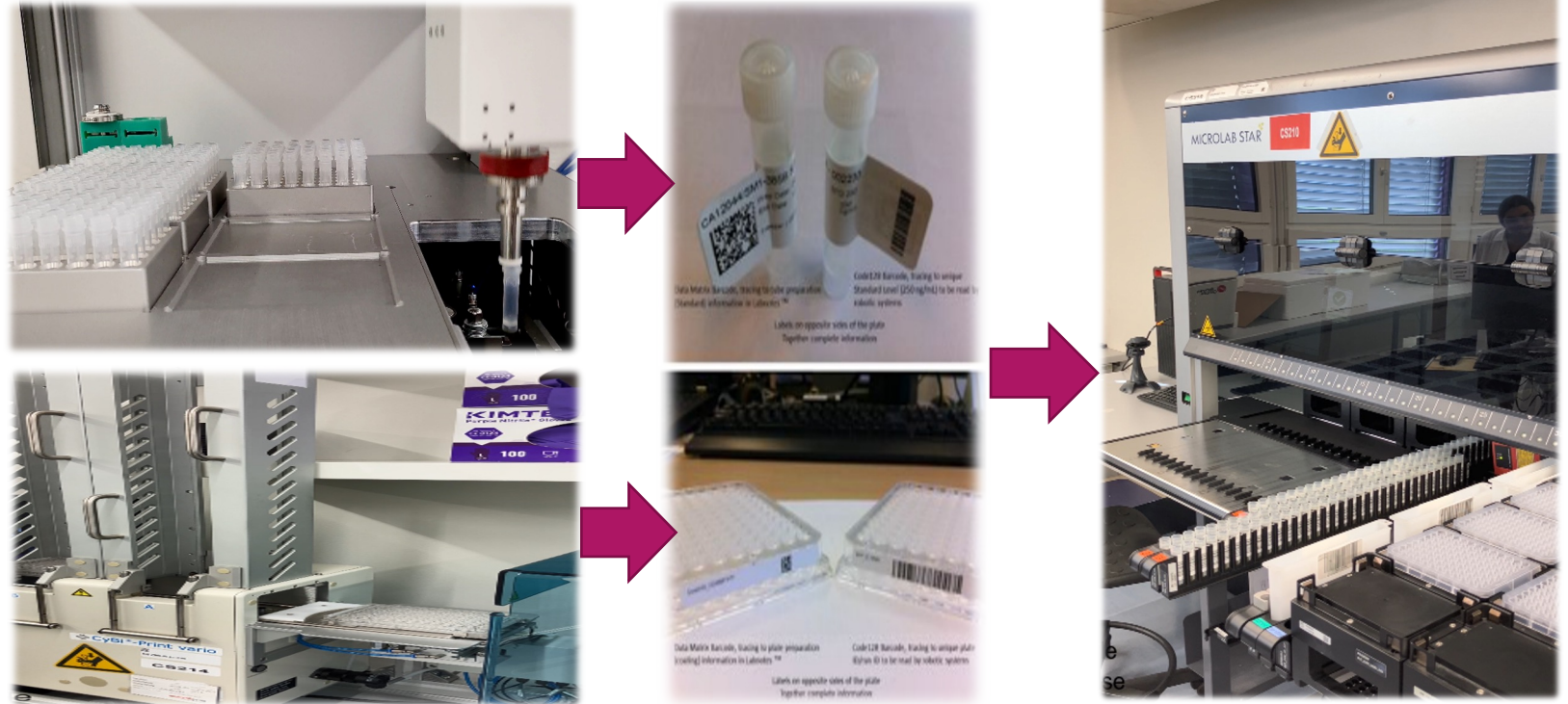
Plates labelled with Print vario (Analytik Jena) with Run ID and ELN ID
