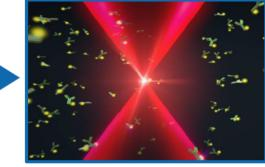
Digital counting of molecules as they pass through interrogation space: Low level background "thresholded" out
