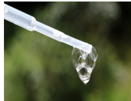
Froth formation during pipetting leads to measurement errors
