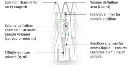
Hydrophobic barriers stop liquid flow – ensures consistent volume delivery and facilitate parallel processing
